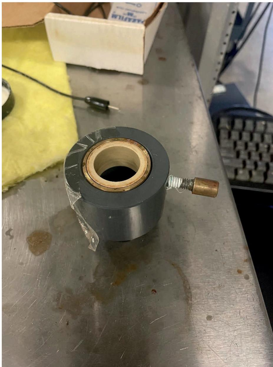
Figure 94. PVC Experimental Apparatus for Use in OCP Calibration
