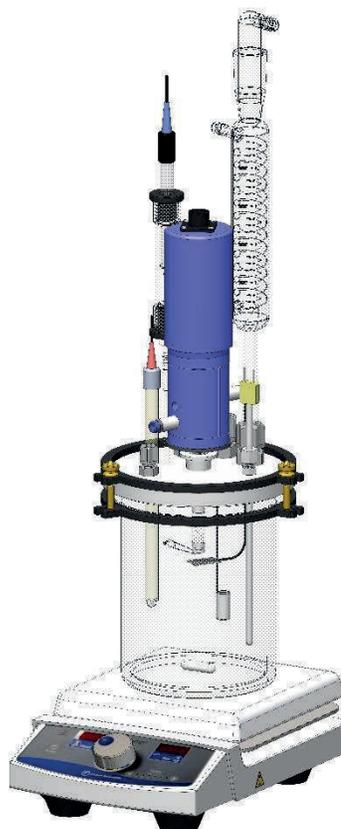
Figure 6. 1 L glass cell set up for RDE experimentation (Cody Shafer)
