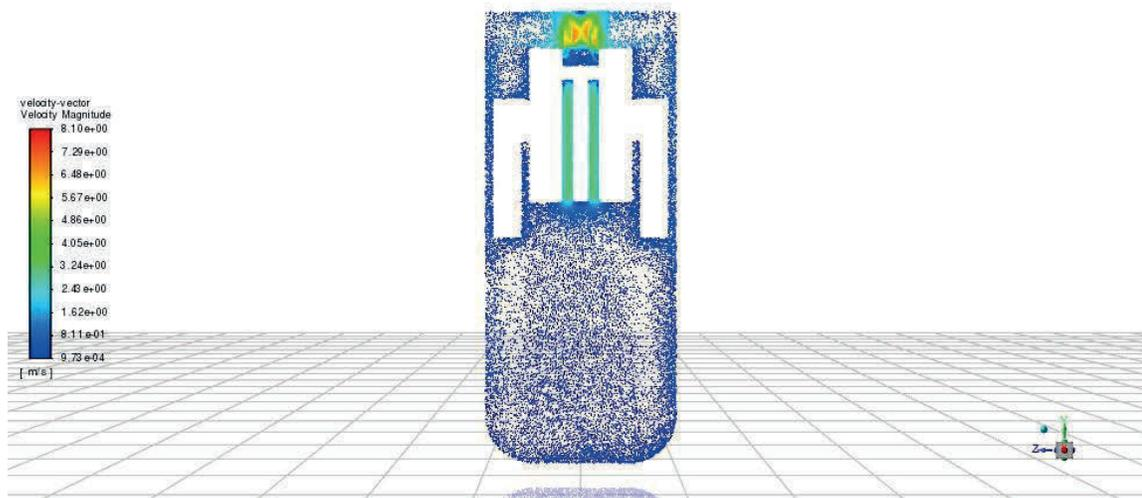
Figure 71. Velocity vectors in yz cross-section of model without internal flow straightener at 5000 RPM impeller speed
