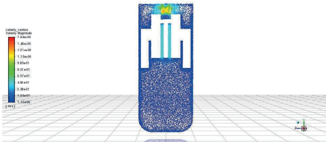
Figure 63. Velocity vectors in yz cross-section of model without internal flow straightener at 1000 RPM impeller speed
